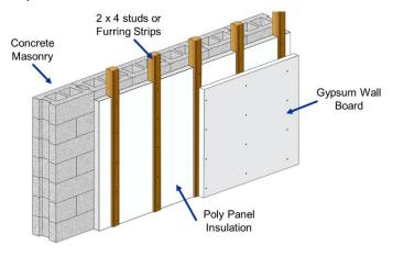
Code Approvals: Underwriters Laboratory Listed, UL ER7260, for interior and walls. Please consult local building codes for system requirements and modern basement moisture management building techniques. Insulation must be separated from living areas by an approved thermal barrier of 0.5-inch gypsum wallboard or equivalent.
